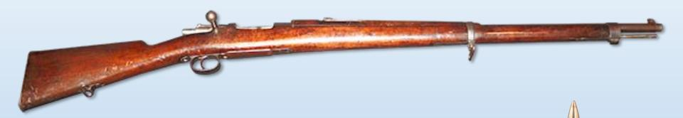
TYPE: BOLT ACTION RIFLE COUNTRY OF ORIGIN: GERMANY OPERATION: BOLT ACTION CALIBER: 7MM MAUSER MODEL YEAR: 1893
