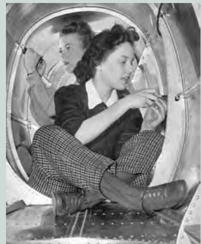
Left: Women workers install fixtures and assemblies to a tail fuselage section of a B-17 bomber. Above: Production Aids for the Grumman Aircraft Engineering Corporation.
