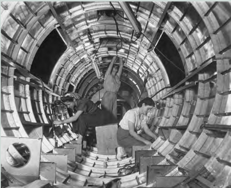
Left: Women workers install fixtures and assemblies to a tail fuselage section of a B-17 bomber. Above: Production Aids for the Grumman Aircraft Engineering Corporation.
