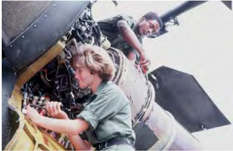
Servicing the Engine of a CH-47 Chinook Helicopter
